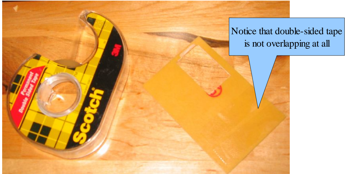
Preparing the circuit board for machining
